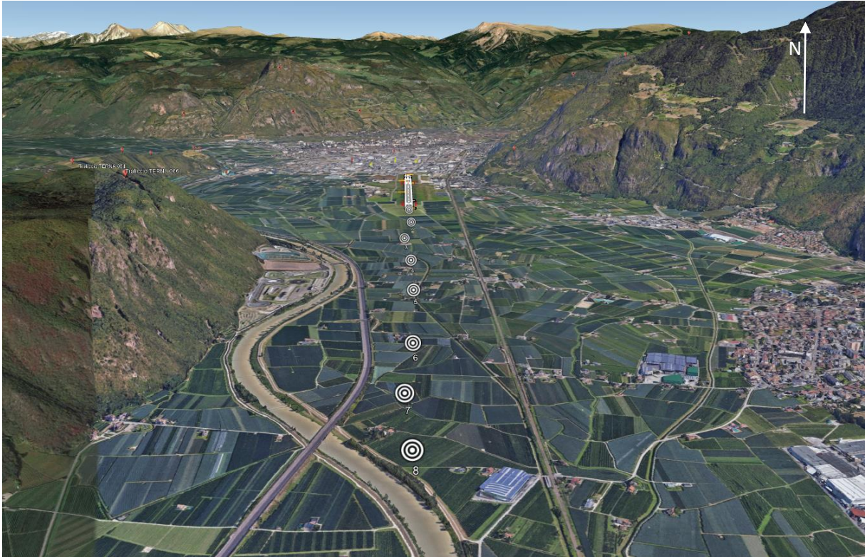
Figure 9: Lead-In sequenced flashing lights – day
